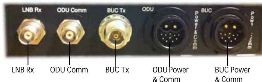
Figure 4-5: Connectors on the rear side of the antenna
