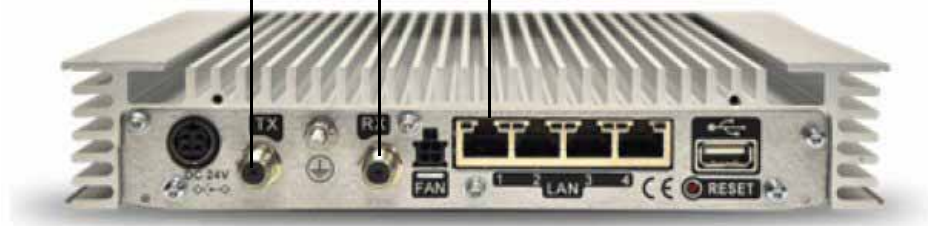
Figure C-7: Connecting Newtec MDM3100 to the ACU (OpenAMIP)
