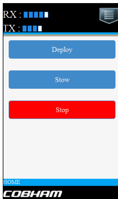
Figure 2-8: Mobile web interface, for basic operation
