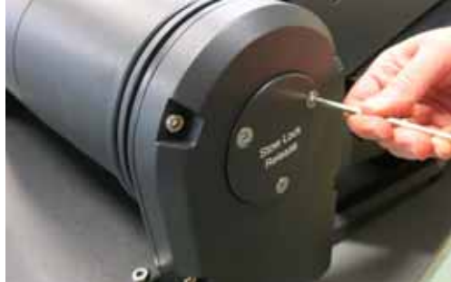
Figure 7-4: Covers for manual elevation adjustment and stow lock release
