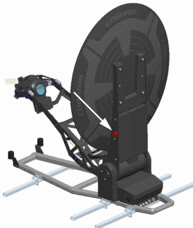
Figure 4-7: Emergency stop button
