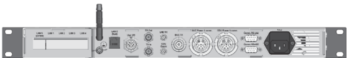
Figure 4-1: ACU connector panel overview
