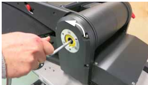
Figure 7-6: Manual elevation adjustment
