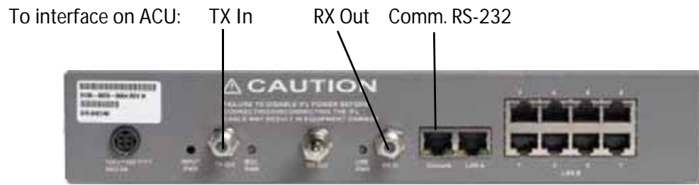
Figure C-10: Connecting iDirect iNFINITI 5000 series to the ACU (Serial)
