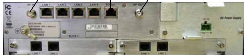
Figure C-20: Connecting Gilat SkyEdge II VSAT modem to the ACU
