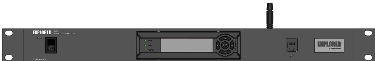
Figure 2-7: ACU front panel
