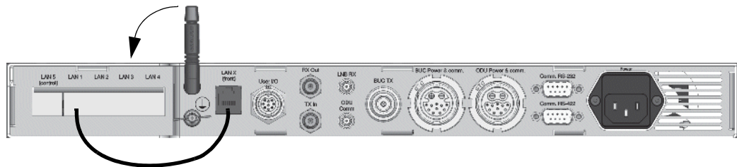
Figure 3-2: ACU connector panel with WLAN antenna
