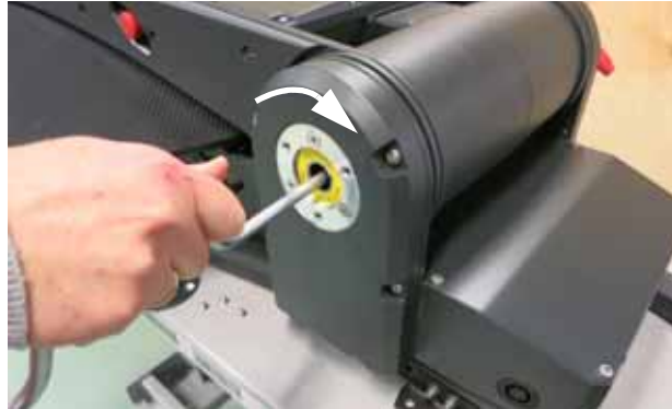
Figure 7-8: Manual elevation adjustment
