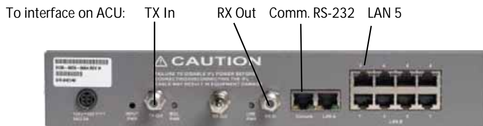
Figure C-1: Connecting iDirect iNFINITI 5000 series to the ACU (OpenAMIP)
