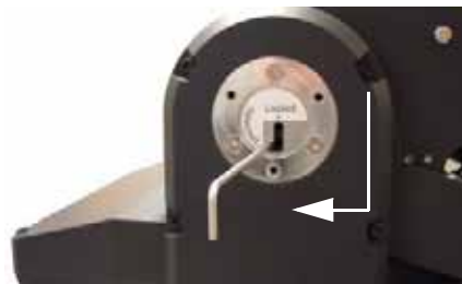
Figure 7-5: Stow lock release
